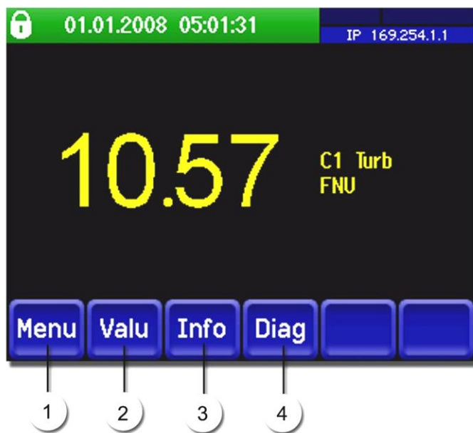
Figure 7: Control components in normal operation
